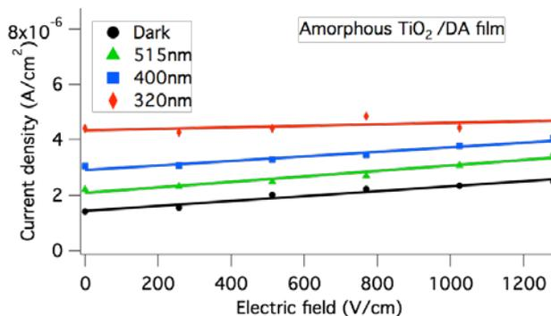
Figure 3. Current density vs. electric field spectra from amorphous TiO<sub>2</sub>/DA film.
