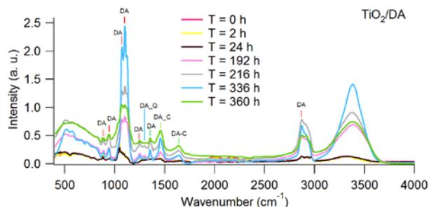
Figure 2. IR spectra for amorphous TiO<sub>2</sub>/DA sample as KBr pellets.
