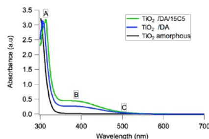
Figure. Absorption spectra of the TiO<sub>2</sub>/DA (blue line) and TiO<sub>2</sub>/DA/15C5 (green line) films. The spectrum for amorphous film corresponds to the black line.
