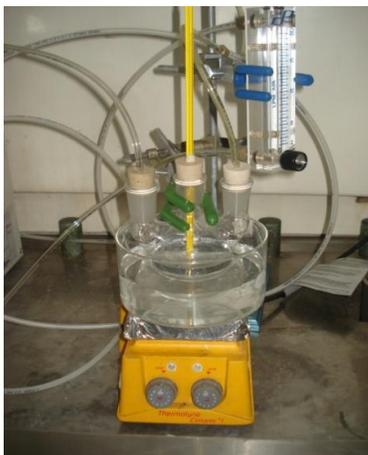
**Figure 12.** Set-up for synthesis of PMMA spheres.
