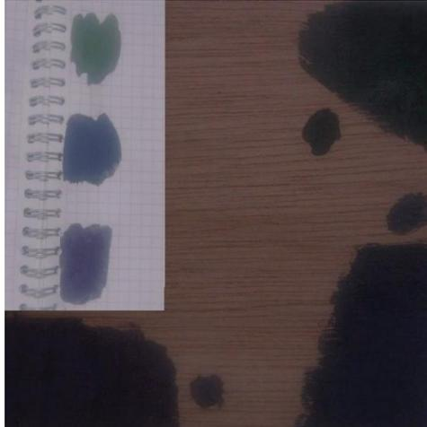
**Figure 22.** Paint resulted of a mixture of D.I. water, solution based on polyvinyl acetate and the colored powders. Photograph of paint applied on different surfaces, i.e., paper and wood.
