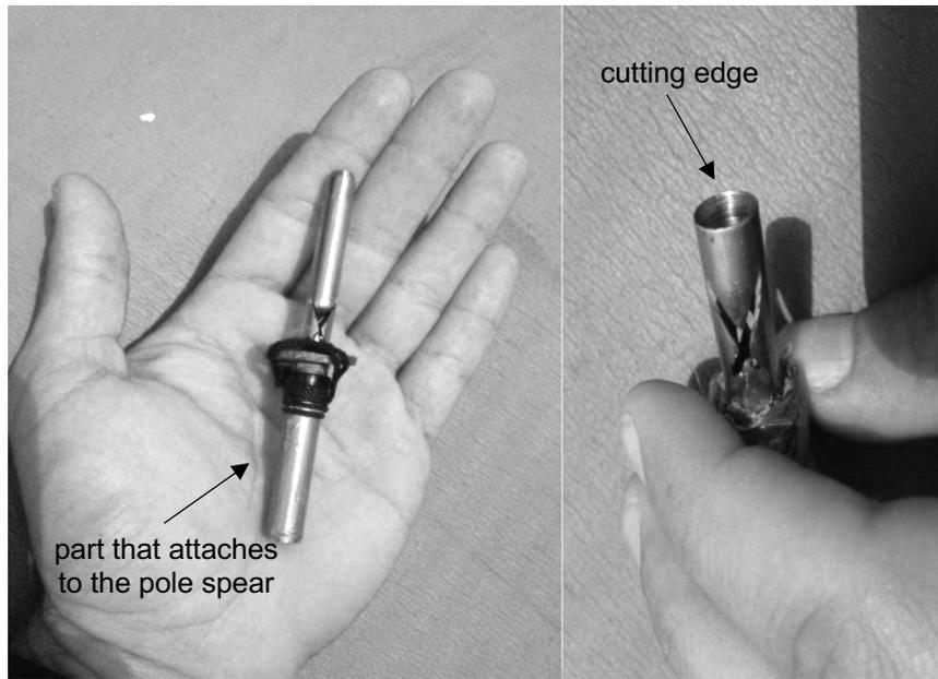
**Figure 3.** Stainless steel biopsy darts used for NES sampling
