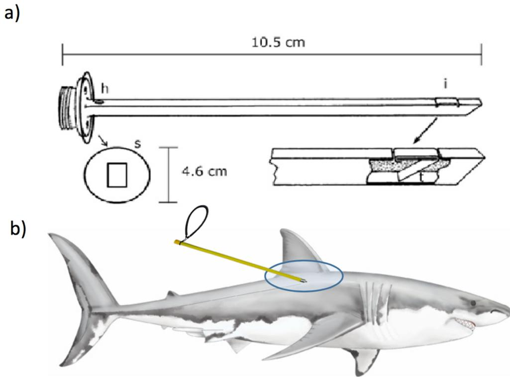
**Figure 2.** (a) Diagram of the biopsy dart used for WS sampling, (b) Sampling area
