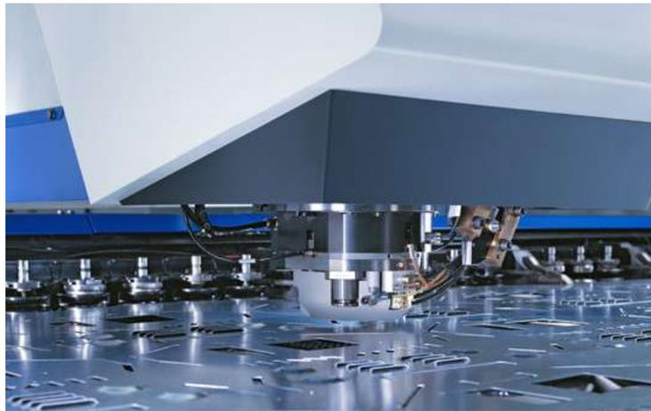
Figura 8. Vista del carro portaherramientas de la Trupunch de Trumpf (fuente: [http://www.trumpf.com/scripts/redirect2.php?domain=http://www.trumpf.com/&nr=1&content=1.stanzmaschinen TruPunch-5000 v2.html](http://www.trumpf.com/scripts/redirect2.php?domain=http://www.trumpf.com/&nr=1&content=1.stanzmaschinen%20TruPunch-5000%20v2.html), 2-XI-2008)
