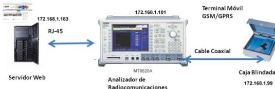
The IP network segment 172.168.1.X was used with a network mask with 24 bits. Table 5.2 shows the IP Addressing scheme used
