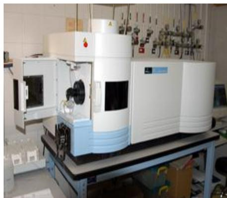
**Figura 8:** ICP-OES Perkin Elmer 4300 DV (Anton Paar Comp.)
