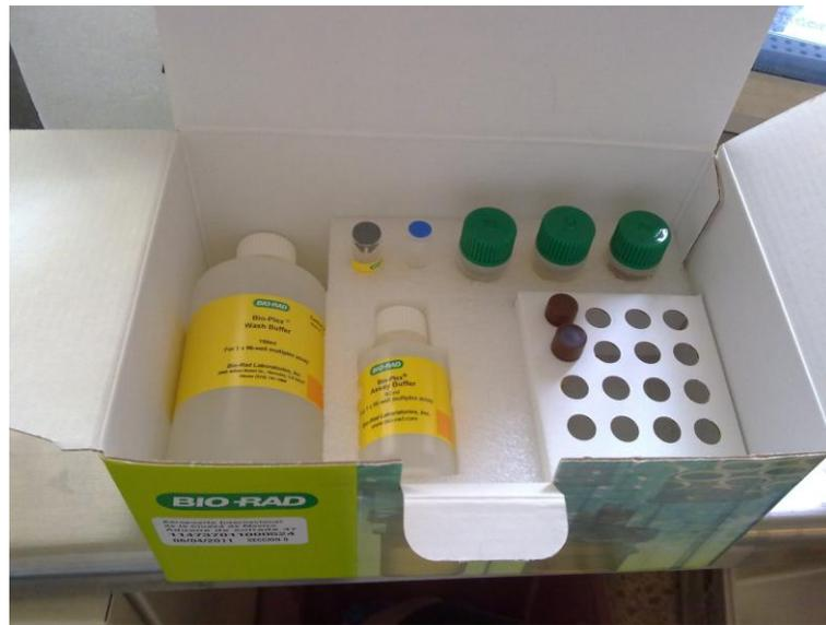
Figura 7. Kit M50-0KCAF0Y de Bio-Plex Pro-Human Cytokine 27-plex Assay de BIO-RAD.
