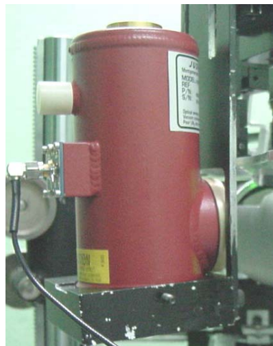
Figura 18. Detector infrarrojo CdTeHg, EG&G Judson Model J15D2-M204-S01M.
