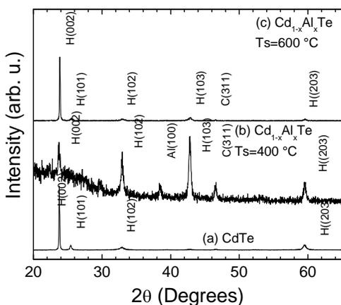
**Figure 2.** Representative X-ray diffractograms for (a) CdTe film, (b)  $\text{Cd}_{1-x}\text{Al}_x\text{Te}$  films deposited at  $T_s = 400^\circ\text{C}$  and (c)  $\text{Cd}_{1-x}\text{Al}_x\text{Te}$  films deposited at  $T_s = 400^\circ\text{C}$ .
