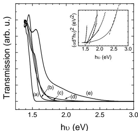
**Figure 3.** Room temperature transmission spectroscopy spectra for samples deposited at  $T_s = 400^\circ\text{C}$ . (a) sample CMT5, (b) CMT9, (c) CMT3, (d) CMT8 and (e) CMT7. The inset corresponds to the fitting of the transmission spectra to the model of direct transitions between parabolic bands.
