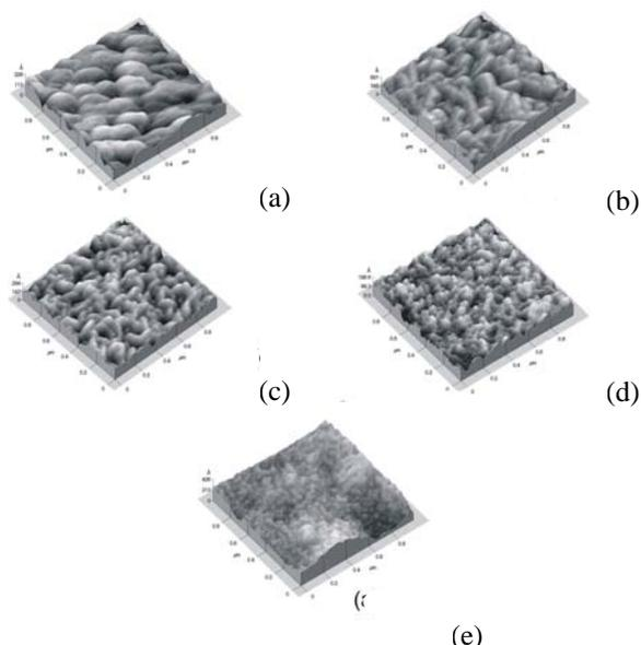
**Figure 1.** Atomic force micrographs for samples deposited at  $T_s = 400^\circ\text{C}$ . (a) CMT8, (b) CMT9, (c) CMT7, (d) CMT3 and (e) CMT5.
