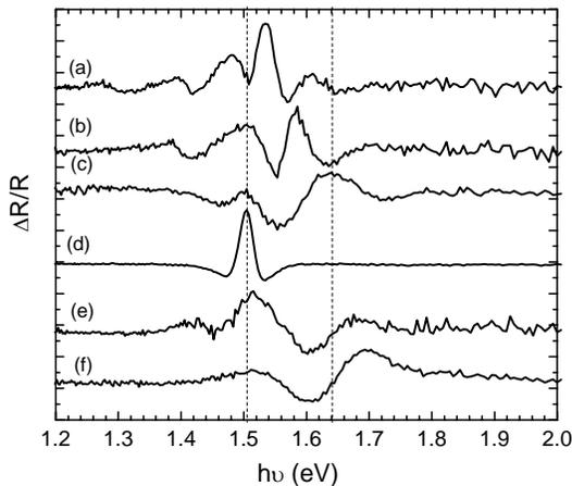
**Figure 5.** Room temperature photoreflectance spectroscopy for samples grown at  $T_s = 400\text{ °C}$ : (a) CMT9, (b) CMT8 and (c) CMT7; and grown at  $T_s = 600\text{ °C}$ : (d) CdTe thin film, (e) MY9 and (f) MY6. The fitting to the theoretical model is shown with circles. Broken lines are just a guide to the eye.
