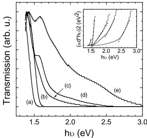
**Figure 4.** Room temperature transmission spectroscopy spectra for samples deposited at  $T_s = 600\text{ °C}$ . (a) polycrystalline CdTe sample, (b) MY1, (c) MY5, (d) MY9 and (d) MY6. The inset corresponds to the fitting of the transmission spectra to the model of direct transitions between parabolic bands.
