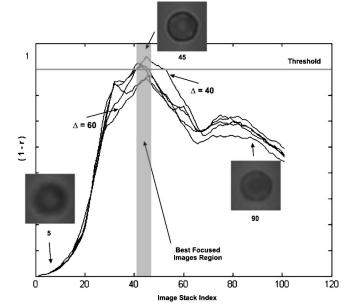
**Fig. 5** Dark-field curves of 1 - r with  $\Delta = 40$  to 60 pixels, showing the best-in-focus image and its index from the captured image stack.
