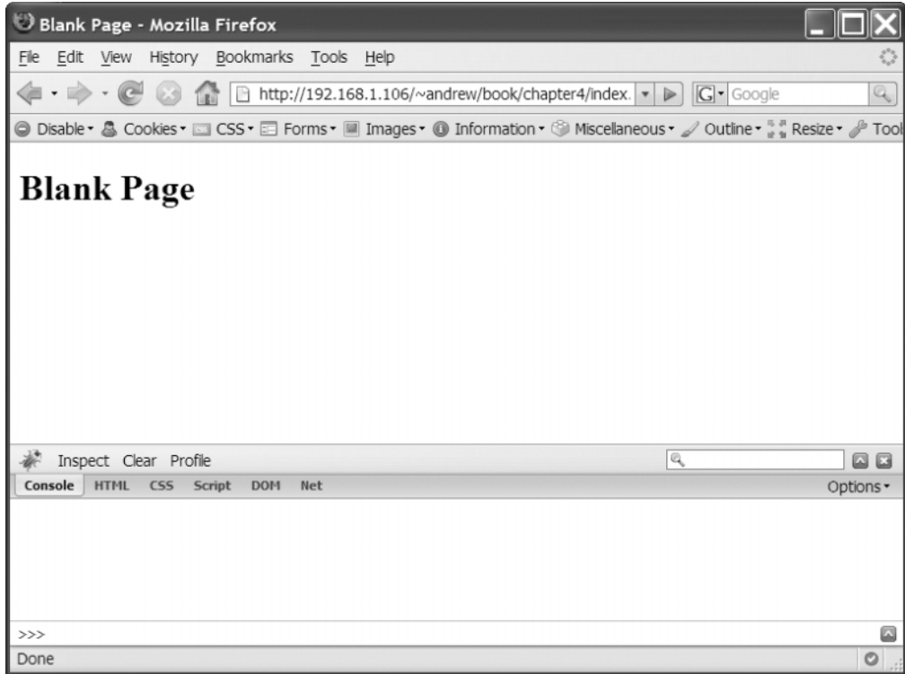
Figure 4-1. Firebug is open to the console tab at the bottom of the screen.
