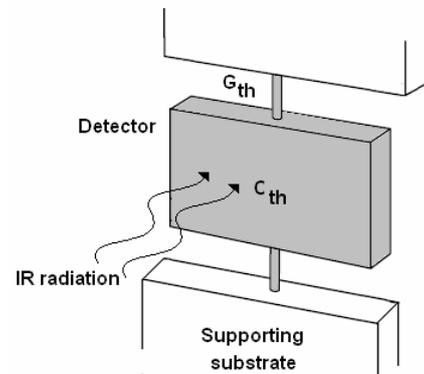
Fig. 1 Simplified bolometer layout.
